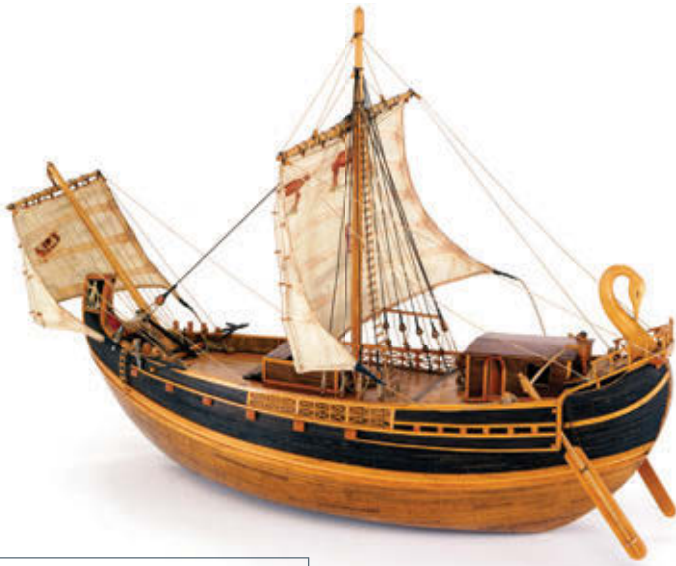
Source 4.59 Roman merchant vessels were powered by sails and had deep hulls to maximise cargo space.
