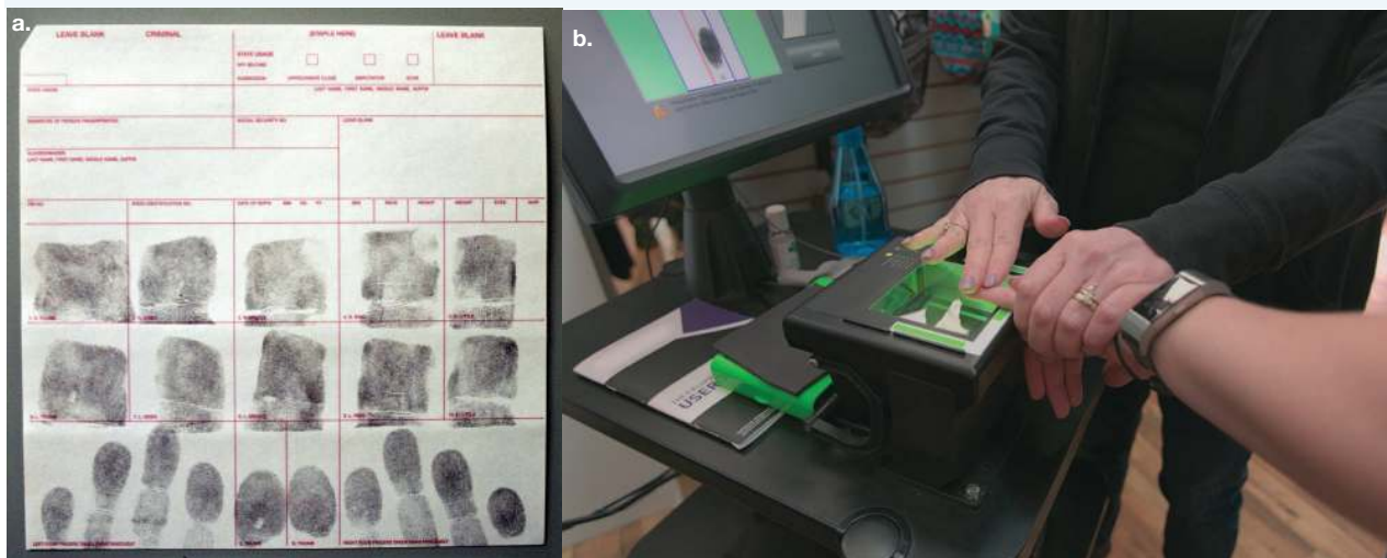
FIGURE 11.14 a. Both rolled and flat fingerprints are taken in crime investigations. b. Electronic fingerprint scanners similar to this are now used to record fingerprints.
