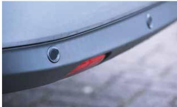
FIGURE 8.13 Sonic motion detectors are used on the bumpers of cars to help the driver detect the distance between the car and another object.
