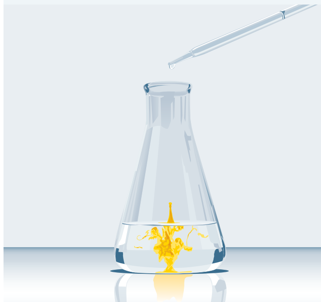
FIGURE 5.24 The formation of the brilliant yellow precipitate, lead iodide, from the colourless solutions of lead nitrate and potassium iodide
