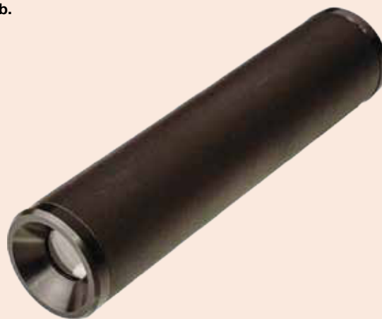
FIGURE 4.26 a. Design of Bunsen's original spectroscope and b. a modern version of a spectroscope, similar to that found in many school laboratories
