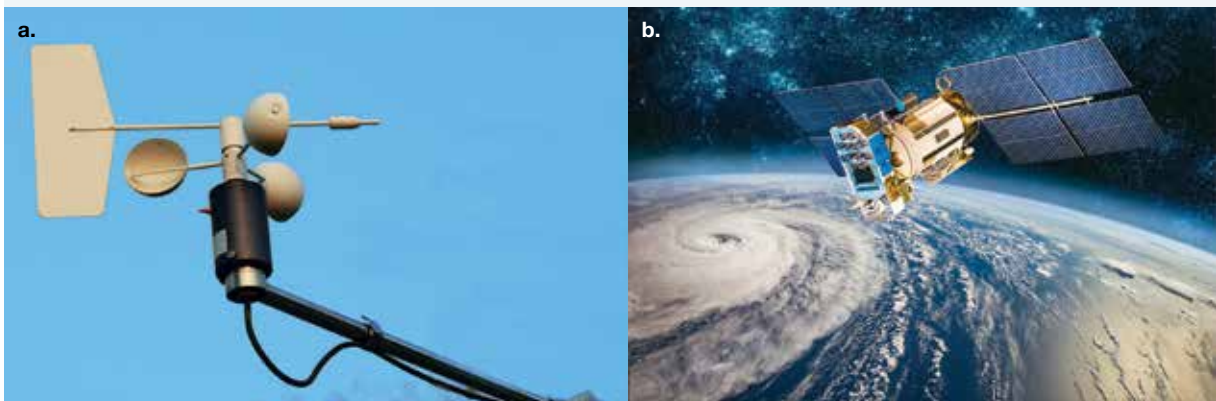
FIGURE 7.20 a. Weather stations contain devices such as a thermometer to measure temperature, a barometer to measure atmospheric pressure, a hydrometer to measure humidity, an anemometer to measure wind speed and a wind vane to measure wind direction. b. Some of this information can also be collected from space, using satellites to monitor weather from Earth's orbit.
