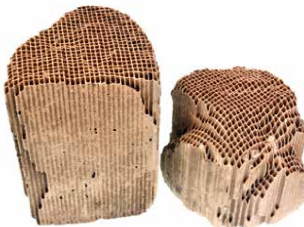
FIGURE 5.34 The honeycombed surface of catalytic converters helps to maximise their surface area and help convert harmful gases into harmless ones.
