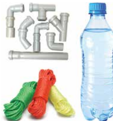
FIGURE 5.40 Polymer materials: PVC pipes, polyethylene bottle and nylon rope
