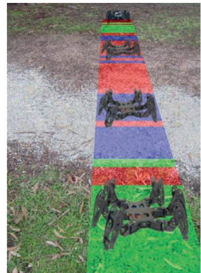
Figure 3.1.17 When the terrain detection algorithm was implemented in ROS software, this terrain was classified as a combination of grass (green), rocks (blue) and mulch (red).
