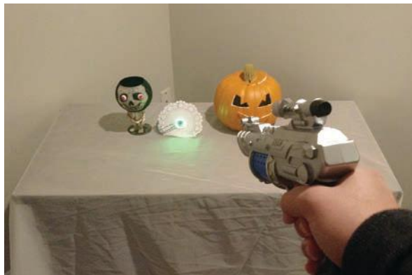
Figure 3.2.24 This IoT project showcased on hackster.io uses Particle Photon and Adafruit trinket microcontrollers to build a homemade laser tag game that dispenses lollies.
