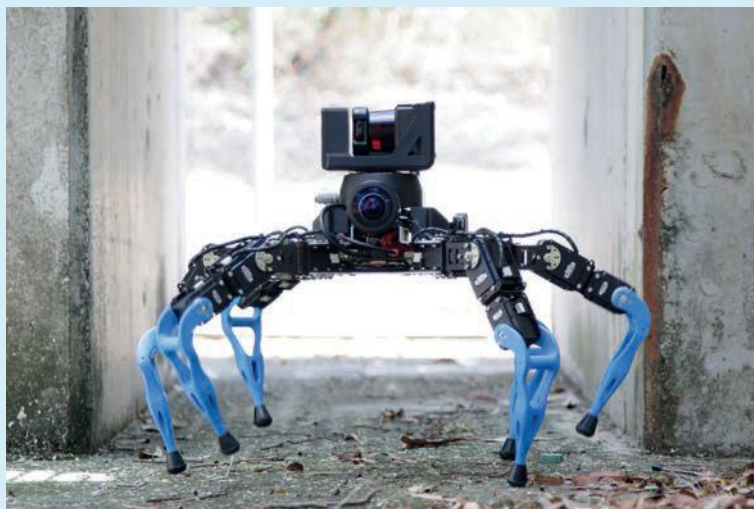
Figure 3.1.13 Legged robots can climb over obstacles more easily than wheeled robots.
