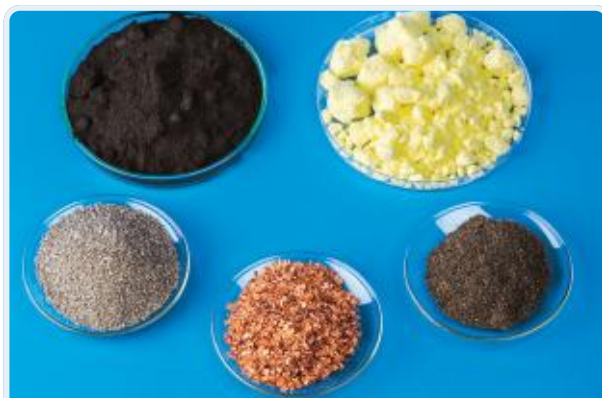
FIGURE 9.2.3 One mole each of five different substances. The mass of 1 mol varies depending on the substance.
