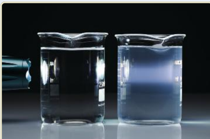
FIGURE 6.2.10 The experimental set-up to classify clear liquids
