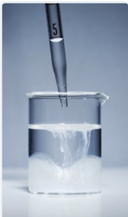
FIGURE 8.3.3 Both silver nitrate and sodium chloride are clear aqueous solutions. When mixed, a white precipitate of silver chloride is formed, which eventually settles on the bottom of the beaker.
