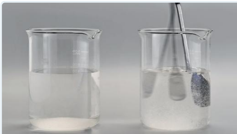
FIGURE 19.3.3 Stirring has the same effect as increasing the surface area because more particles are exposed to one another.
