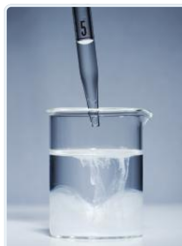
FIGURE 15.1.2 A silver chloride precipitate forms when solutions of sodium chloride and silver nitrate are mixed.
