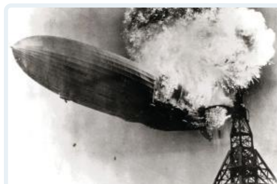
FIGURE 6.1.2 The Hindenburg disaster occurred because early airships were filled with light, but flammable, hydrogen.
