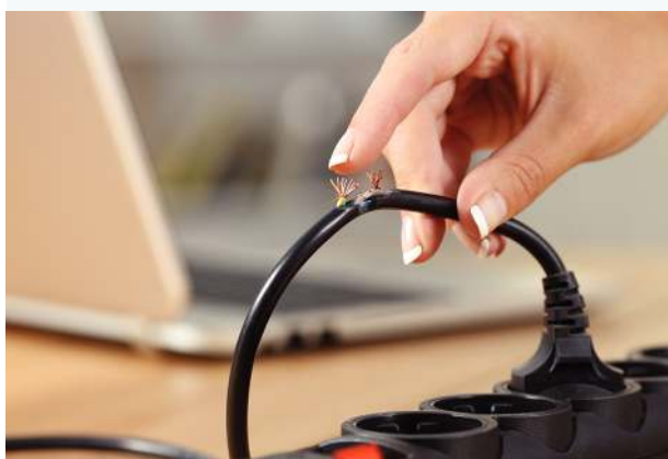
FIGURE 5.13 Frayed electrical cords
