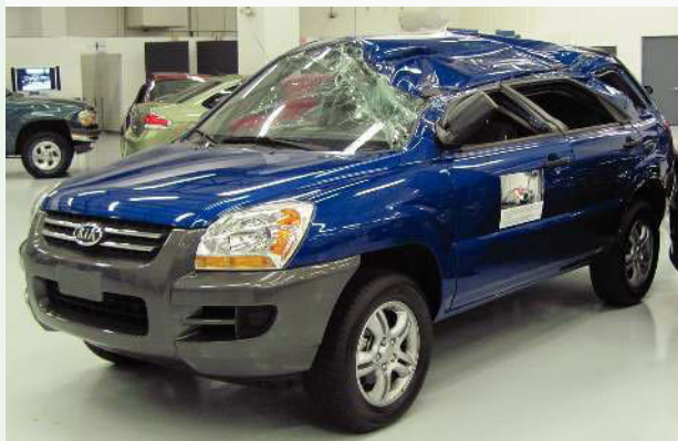
FIGURE 10.27 A vehicle that has undergone a roof crush test
