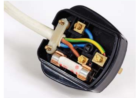
FIGURE 5.16 A three-pin plug with its back cover removed. The earth wire is covered in a green and yellow coating. Also note the cartridge fuse inside the plug.
