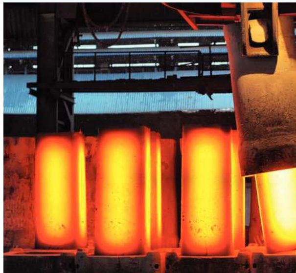
FIGURE 1.9 This steel is nearly 1000 °C and has recently been poured into a mould to shape it. The steel will continue to glow until it has cooled to about 400 °C.
