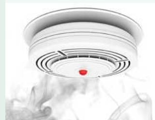
FIGURE 7.18 Smoke alarms are set off when smoke blocks the path of alpha particles
