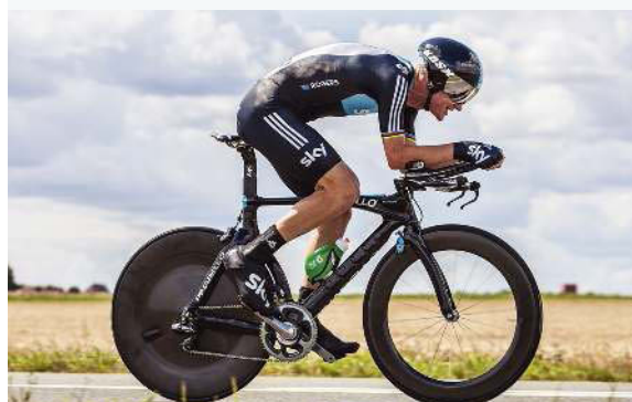
FIGURE 10.5 Racing cyclists reduce the effects of fluid friction (air resistance) by wearing streamlined costumes and using aerodynamically designed bicycles.
