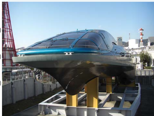
FIGURE 3.19 The world's first superconducting, magneto-hydrodynamically propelled vessel, the Yamato 1, launched in 1991
