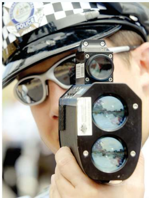
FIGURE 8.5 The radar gun would measure a different speed if it was in a moving vehicle.
