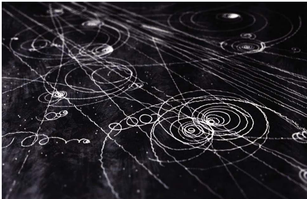
FIGURE 3.1 Cloud chambers reveal the paths of charged particles produced in radioactive decay. A combination of magnetic and electric fields allows the tracks to be linked to particles with particular charge, mass and velocity, giving clues to the identity of the products.
