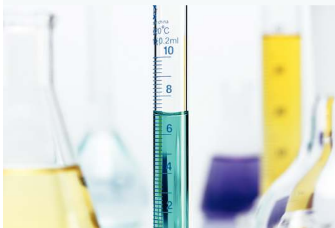
FIGURE 13.44 Reading a measuring cylinder can result in errors
