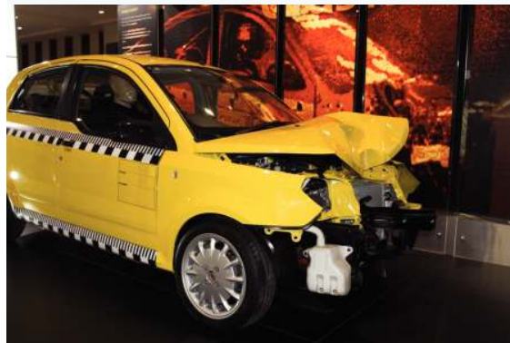
FIGURE 7.2 Cars are designed to crumple in collisions. This increases the time interval over which the momentum changes, decreasing the average net force on the car.
