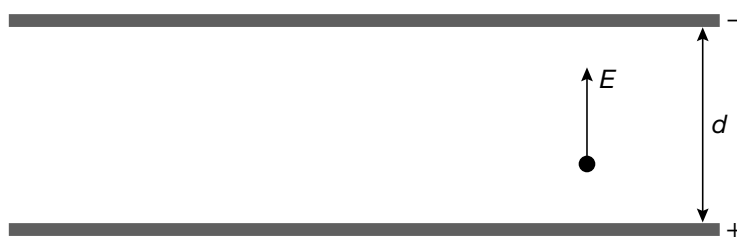
FIGURE 11.3 An electric field set up between two parallel plates connected to a battery
