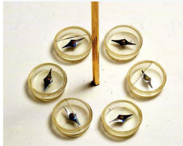
FIGURE 1.37 Magnetic field measurements around a current-carrying wire
