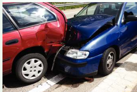
FIGURE 7.14 Crumple zones at the front and rear of cars absorb energy and reduce the magnitude of acceleration during an accident.
