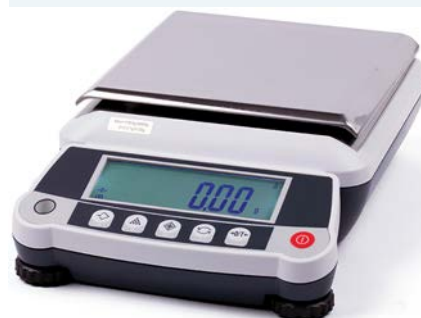
FIGURE 13.46 Top-loading balances measure to a certain number of significant figures
