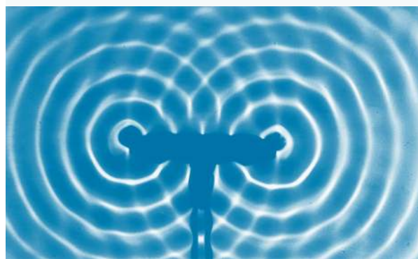
FIGURE 9.18 An interference pattern obtained in water by using two point sources that are in phase
