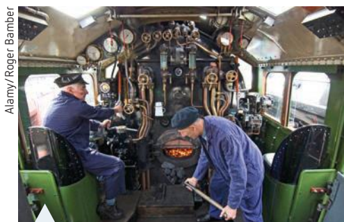
FIGURE 5.1.2 Coal heats the boiler to produce the steam that drives the train engine's pistons.
