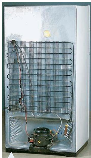
FIGURE 5.3.4 The back of a household refrigerator. The air surrounding the coils is the heat source.
