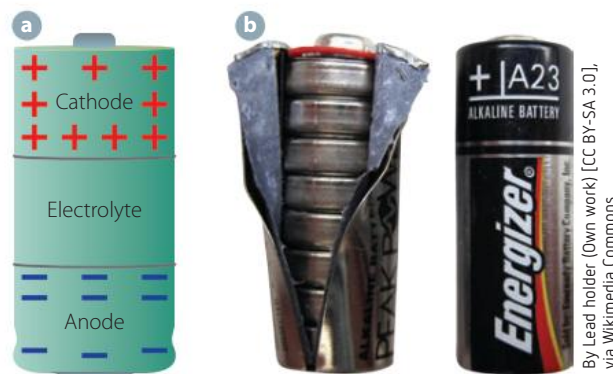
FIGURE 9.3.2 (a) A simplified battery. (b) An AA battery is a collection of smaller cells.
