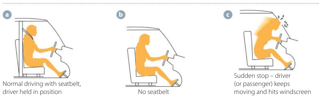
FIGURE 14.6.1 (a) Seatbelts in vehicles enable the occupant to come to a stop with the vehicle. (b) Unrestrained occupants continue towards the windscreen at the speed of the car when the crash begins. (c) A collision with the windscreen can be disastrous.
