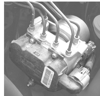
Fig 10.89 Antilock brake systems are closed control systems.
