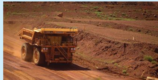
Figure 4.29 An autonomous haul truck drives through a pit at Rio Tinto Group's West Angelas iron ore mine in the Pilbara, Western Australia.
