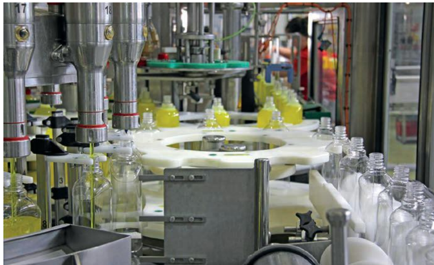
Figure 4.27 Detergent being bottled on an automated production line
