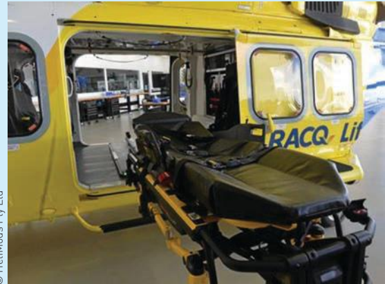
Figure 2.24 HeliMods' automated stretcher system can be used for aircraft and road vehicles. This innovation allows rapid loading of patients at the push of a button.
