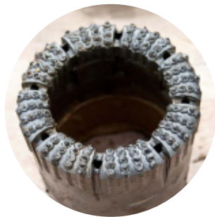
Figure 4.29 A diamond-studded drill bit. These bits tend to be used in mining.
