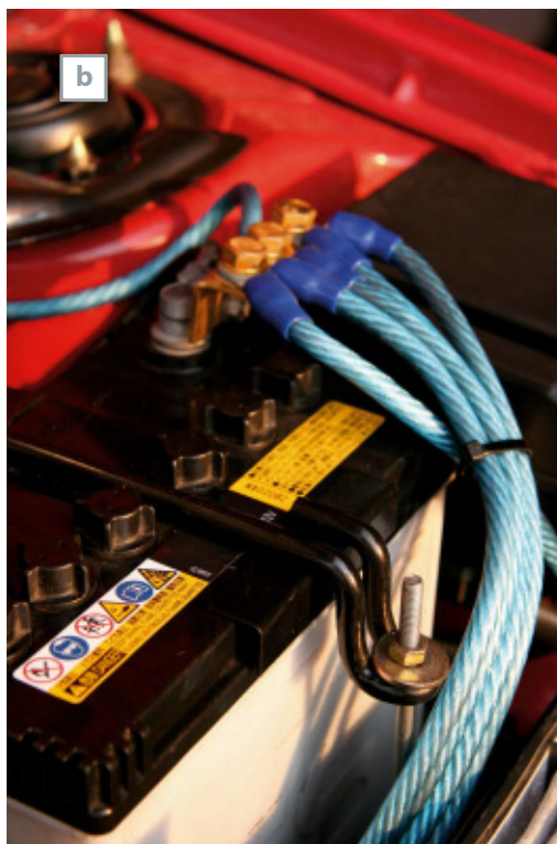
Figure 3.54 Batteries come in all different shapes and sizes, such as (a) everyday batteries and (b) car batteries, but they all transform chemical potential energy into electrical energy.
