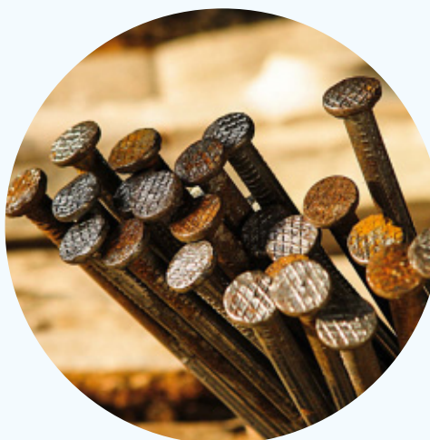
Figure 5.12 Rusting nails can be a problem in structures where they can cause weakness in the structure.
