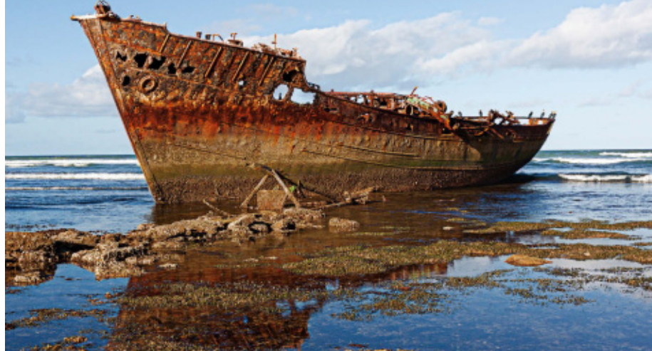
Figure 4.9 The iron of this ship has almost completely corroded.
