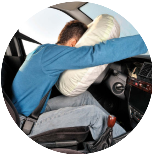
Figure 3.12 Airbags in cars are designed to slow you down before you stop in a crash, reducing the kinetic energy and hopefully preventing injury.
