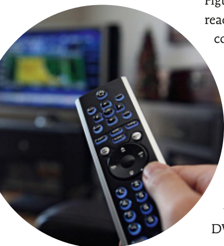
Figure 3.26 A television remote control uses an infrared LED to operate the television.
