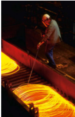
Figure 4.18 Most metals are ductile and can be drawn into a wire.
