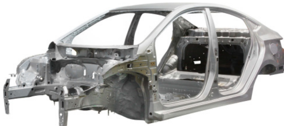
Figure 4.68 The chassis and frame of cars are usually made from steel.
