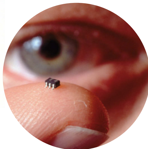
Figure 3.50 When it was introduced in March 1998, this operational amplifier, containing 50 transistors, was the world's smallest integrated circuit. Even smaller integrated circuits are now used in phones, games and many other electronic devices.
