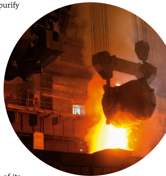
Figure 4.34 Molten iron being poured into a Basic Oxygen Steelmaking furnace.
