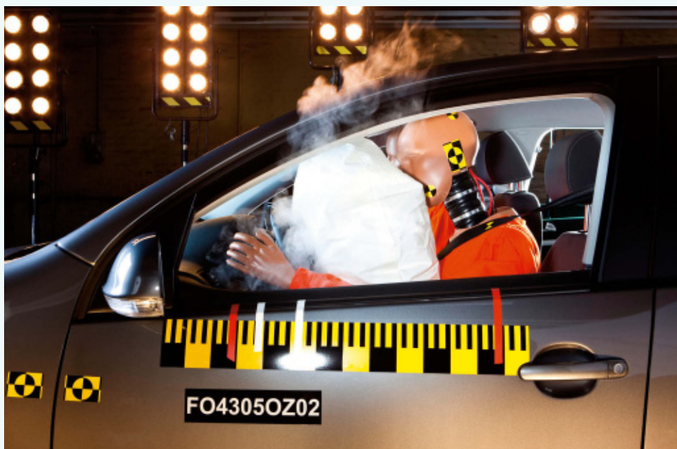
Figure 3.15 Crash test dummies are used to test the safety features of cars.
