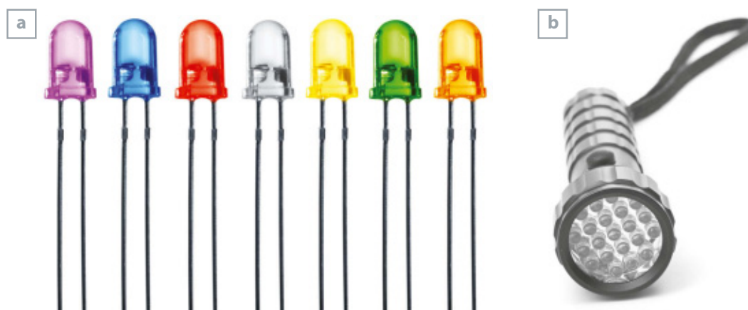
Figure 3.53 (a) Light-emitting diodes (LEDs) are tiny bulbs that use very little energy. (b) LEDs are commonly used in torches.
