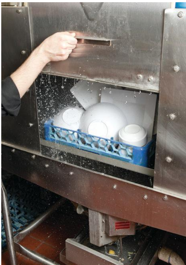
Figure 11.13 Dishwashers should be dismantled for periodic cleaning and maintenance.
