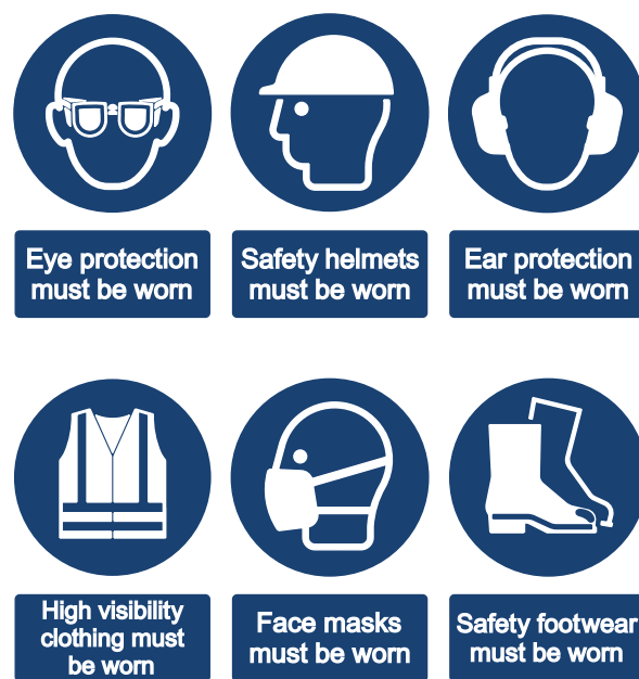
Figure E1.14 PPE signs
