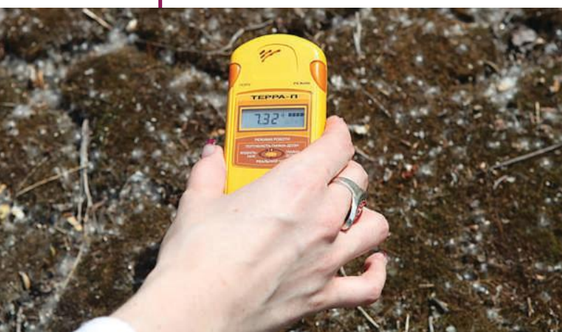
Figure 11.5 Reading the radiation levels with a Geiger counter in front of the reactor in Chernobyl, Ukraine.
