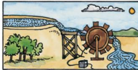
(d) The waterwheel turns a generator to convert mechanical energy into electrical energy.
