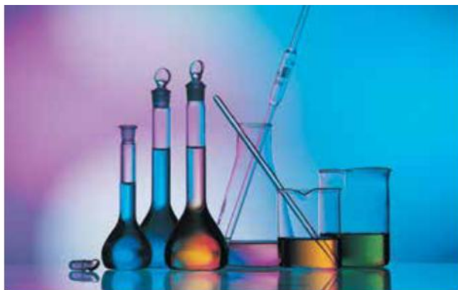
Volumetric flasks, conical flasks, pipettes, burettes and various beakers are used in volumetric analysis.
