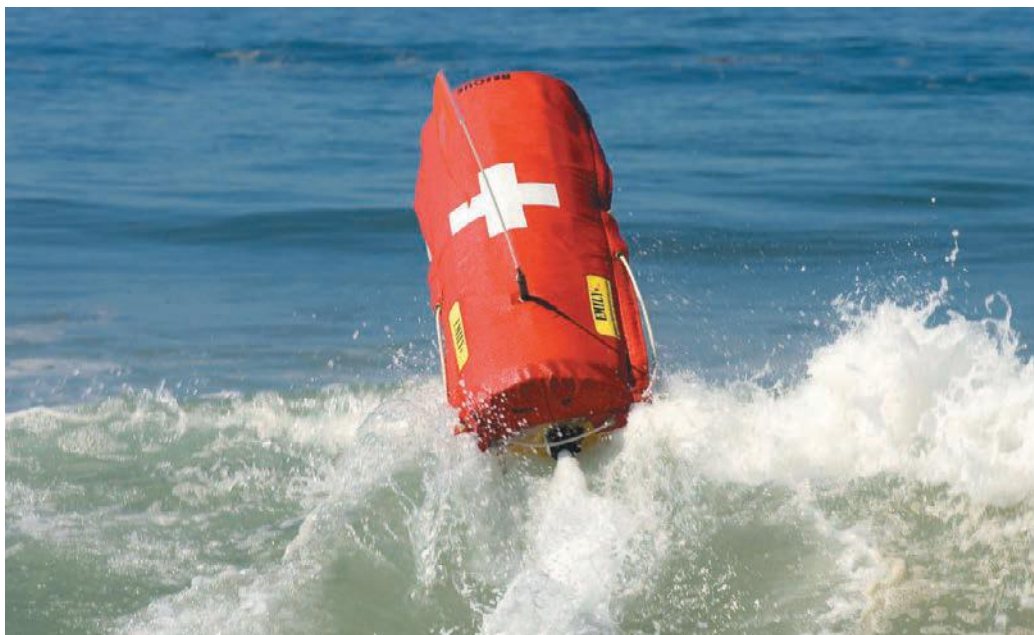
FIGURE 5.10 This mobile robot rescues distressed swimmers by scanning underwater movements with sonar, and enabling lifeguards on shore to provide instructions and reassurance to the person being rescued.
