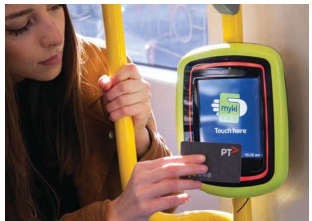
FIGURE 7.15 The myki public transportation ticketing system uses near-field communication to read a commuter's details from their smart card or smartphone.
