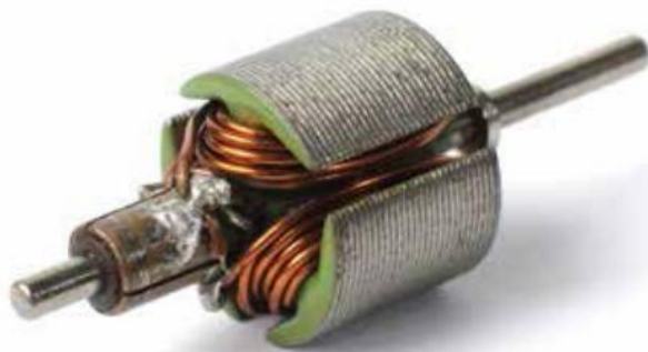
Commutator and coil from a hair dryer
