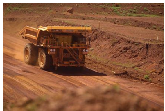
FIGURE 3.2.22 An autonomous haulage truck drives through a pit at Rio Tinto Group's West Angelas iron ore mine in Pilbara, Western Australia.
