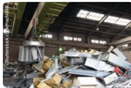
▲ FIGURE 5.7.2 A magnet separates the steel from other recyclable materials.
