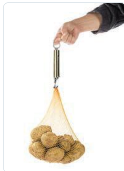
▲ FIGURE 8.2.1 A spring balance measuring the downwards force of a bag of potatoes
