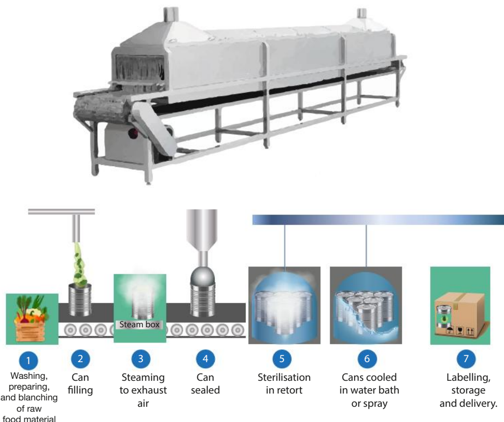
Figure 2.5.3: Exhaust box used in canning (top) and canning process within the exhaust box (bottom).
