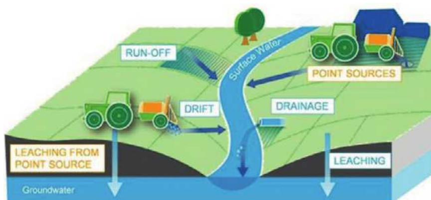
Figure 3.1.15: The movement of pesticides, including run-off, drift and leaching after tractor application.
