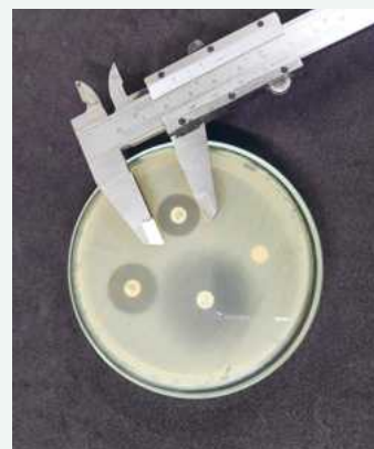
Figure A: Measuring the diameter of a zone of inhibition around a disc dipped in a preserving solution.
