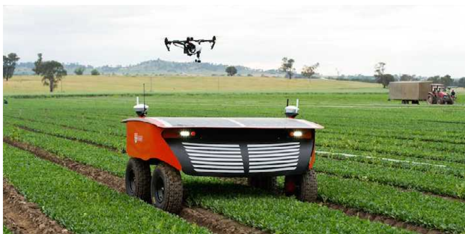
Figure 3.2.2: Australian centre for field robotics (University of Sydney) robot called RIPPA (Robot for Intelligent Perception and Precision Application) for spraying individual weeds with herbicide, and a farming drone monitoring plant health and overseeing RIPPA movements.
