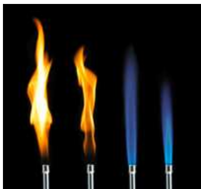
Figure 4.1.4: Bunsen flames produced during complete and incomplete combustion.
