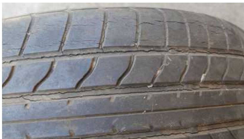
Figure 1.2.7: Car tyres (synthetic polymer) cracking due to ozone exposure.
