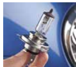
Figure 3.23 Halogen lamps have been commonly used in car headlights and outdoor lighting for decades. The halogen reversibly reacts with a tungsten filament to provide a bright light that also keeps the bulb clean.
