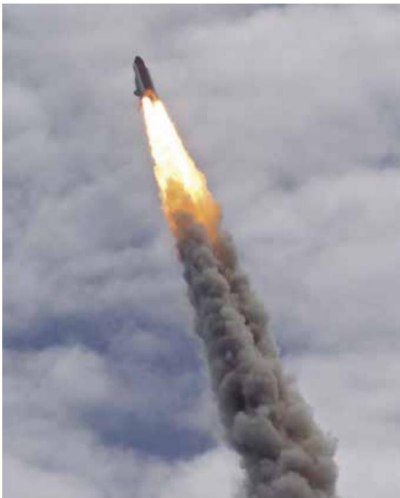
Figure 7.31 The rocket pushes exhaust gases back. As a result the rocket is propelled forwards.
