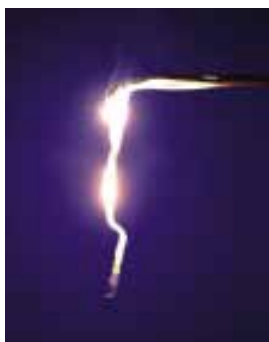
Figure 4.5 The oxidation of magnesium is highly exothermic and produces a very bright flame.
