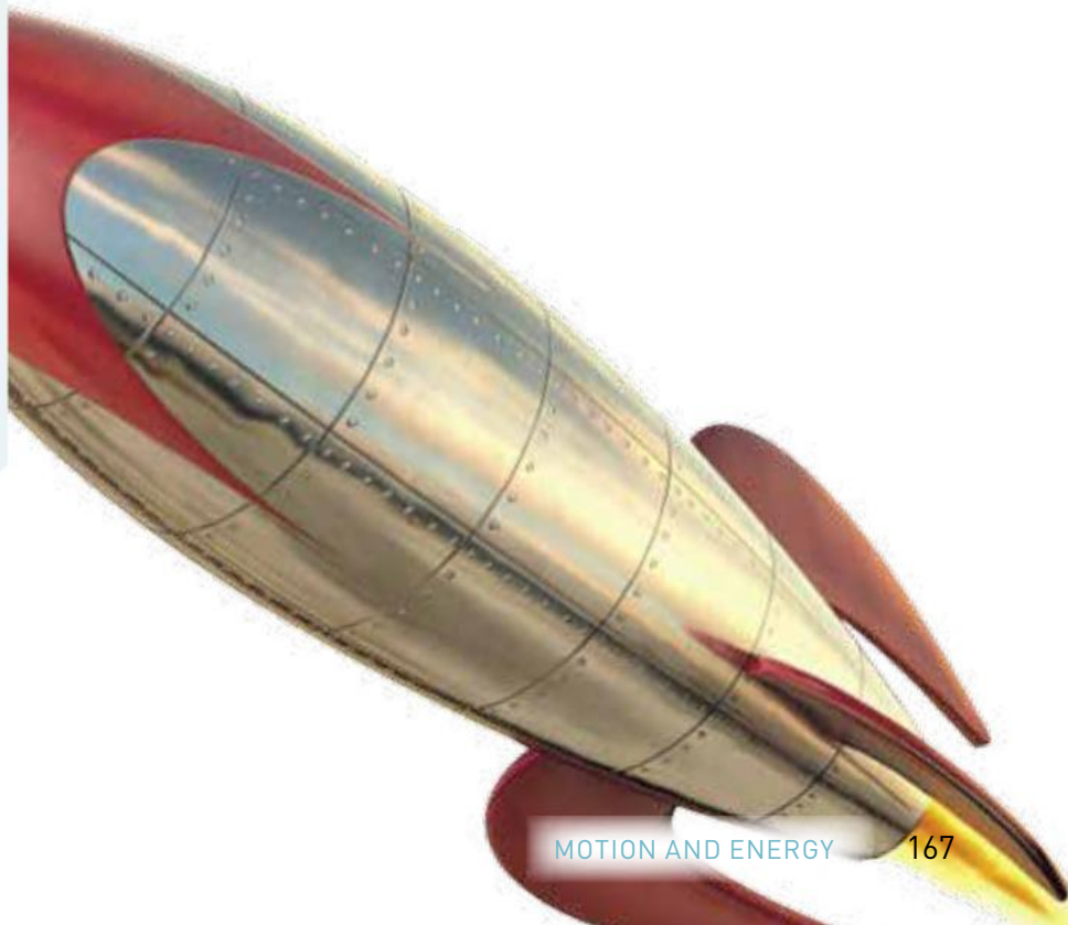
Figure 7.31 The rocket pushes exhaust gases back. As a result the rocket is propelled forwards.
