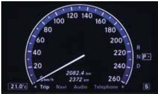
Figure 7.7 A speedometer measures the instantaneous speed of a vehicle.
