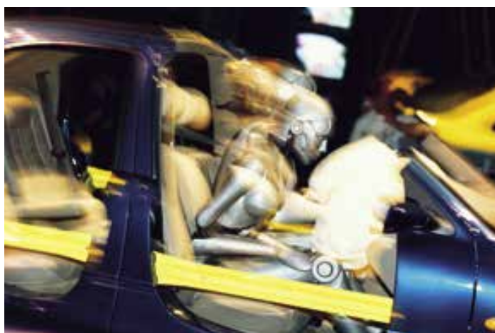
Figure 7.23 Seatbelts are an inertia device. They are often called 'inertia reel seatbelts'. The aim of a seatbelt is to transfer the force on the car to the passenger wearing the seatbelt so that the person moves with the car. You start moving when the car starts moving and, when wearing your seatbelt, you stop moving when the car stops moving.
