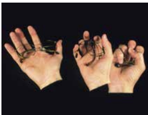
Figure 3.35 Memory wire is useful in eyeglass frames, allowing them to be bent out of shape without breaking.
