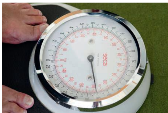
Figure 2.33: The familiar bathroom scale does not measure mass. It measures the force that you exert on it. This force is the weight only when the scale is at rest.
