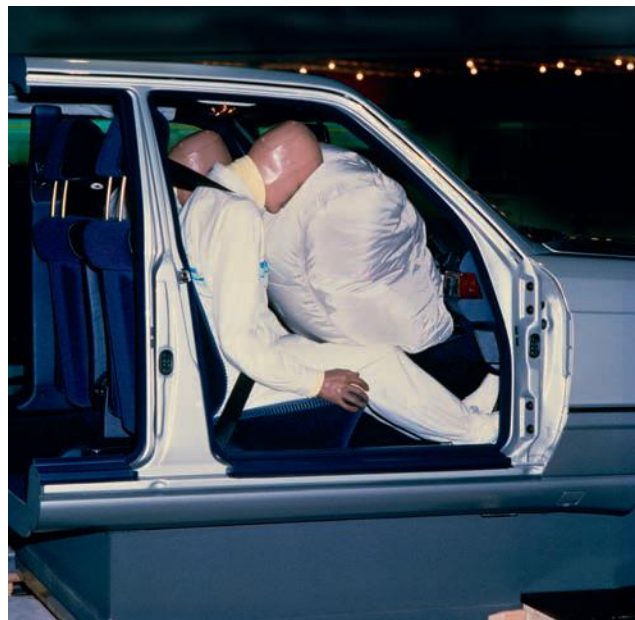
Figure 2.31: The car was originally travelling at high speed. When it hits the wall the car stops, but the passenger wants to stay in the original high speed state of motion. This results in him hitting the steering wheel and the windshield (which is why it is a good idea to have safety belts and air bags).
