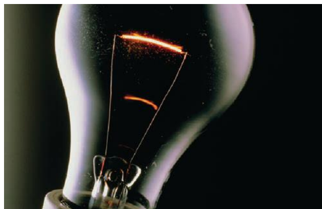
Figure 11.12: The metal filament in a light bulb glows as the current passes through it. It is also very hot. This shows that electrical energy is transferred to both thermal energy and light energy.
