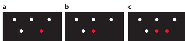
Figure 25.6: The white stars represent the distant background. a The star observed from one position. b The star observed from another position six months later. c The two images are put together to determine the parallax angle. The shift shown here is greatly exaggerated.
