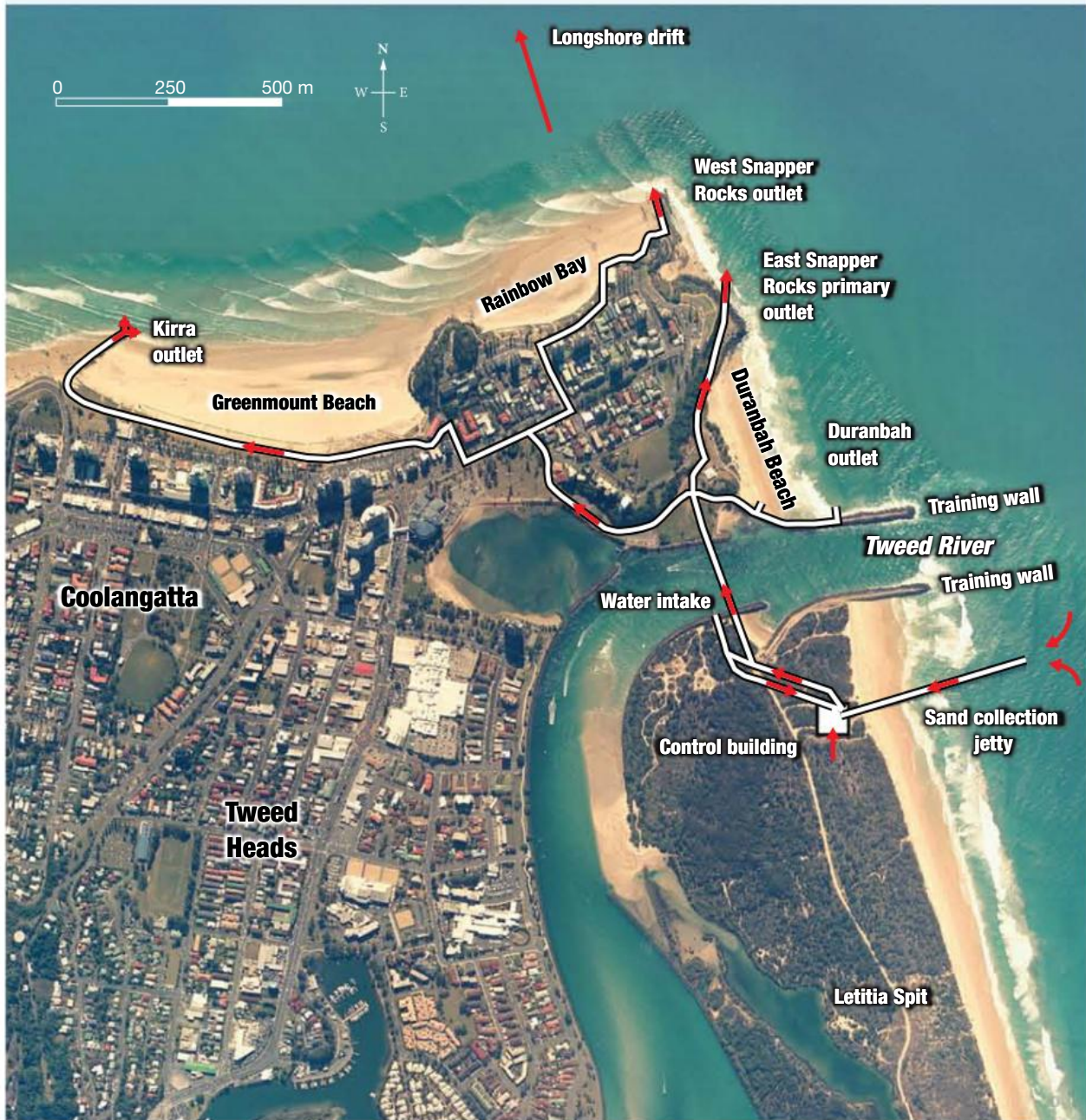
FIGURE 3 Sand bypass system
