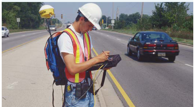
FIGURE 2 Using GPS to survey and record road traffic movements for a local council
