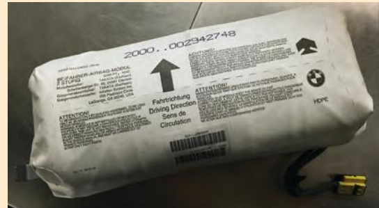
Figure 10.28 A recalled Takata airbag inflator removed from a Honda passenger vehicle. A review panel noted several flawed practices at Takata, including allowing products under development to continue downstream even though design milestones were not met.
