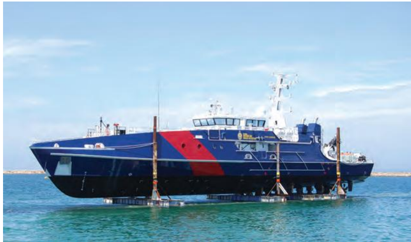
Figure 10.17 Ship builder Austal uses a fixed-position layout in the manufacture of its ships. Here, a Cape Class patrol boat is under construction for the Australian Border Force.
