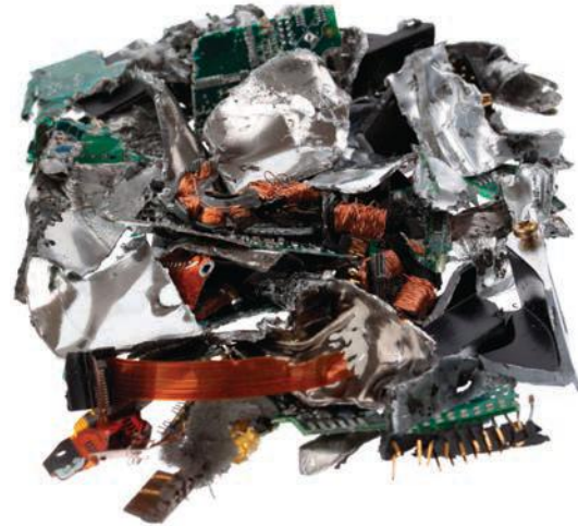
FIGURE 6.21 A hard disk after physical shredding – the ultimate form of disposal
