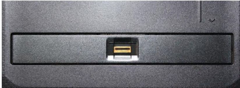
FIGURE 3.40 The fingerprint scanner positioned directly below the trackpad (in-built mouse replacement) on a laptop computer. The user only need run their fingerprint over the brown stripe in the gold section to capture their fingerprint scan.
