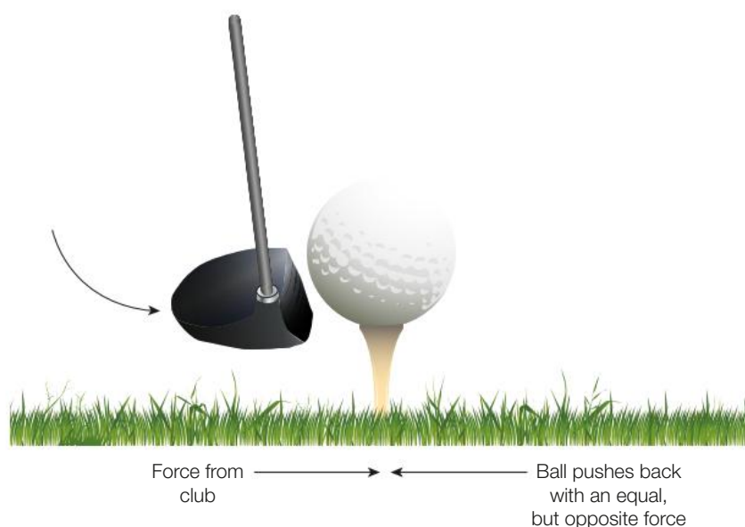
Figure 1.3.16: At impact, the club applies a force to the ball. The ball applies an equal but opposite force back.
