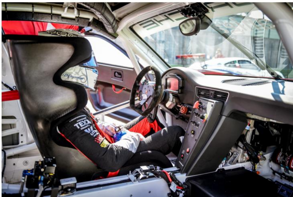
Figure 1.3.15 The interior of a Porsche racing car with only essential instruments and hardware to reduce the car's mass.
