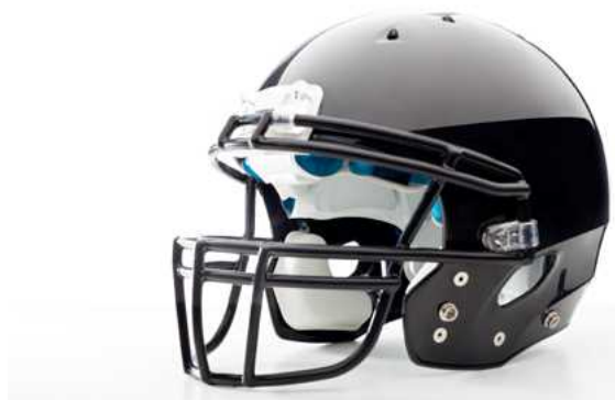
Figure 3.4.4: Traditional American Football helmets were made of a rigid plastic, outer shell. This design limited any ability to 'absorb the impact'. Instead the hard outer shell meant that the time over which the force acted was small. As time and force are inversely proportional to each other in the IMPULSE equation, the force acting on the brain remains high.
