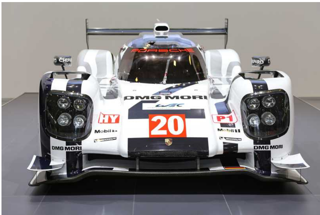
Figure 3.4.1: Carbon fibre body panels make up most of a modern day racing car, as the material is lightweight, yet stronger than steel for its weight.
