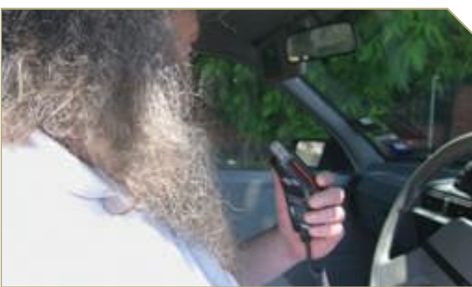
Figure 11.3.4 Alcohol interlock system
