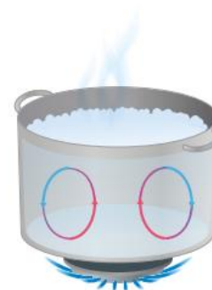
Figure 2 Convection currents are created in a saucepan of water when it is heated. The heated water molecules (shown in red) rise, while the cooler ones (shown in blue) sink.
