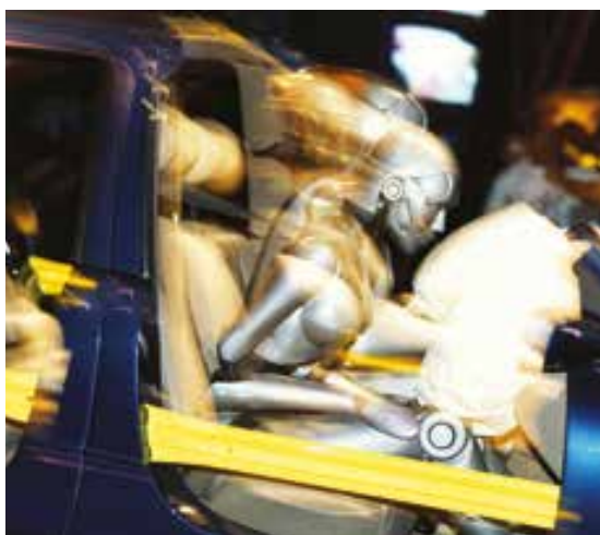
Figure 4 Seatbelts are an inertia device. They are often called 'inertia reel seatbelts'. The aim of a seatbelt is to transfer the force on the car to the passenger wearing the seatbelt so that the person moves with the car. You start moving when the car starts moving and, when wearing your seatbelt, you stop moving when the car stops moving.
