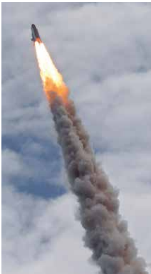
Figure 2 The rocket pushes exhaust gases back. As a result, the rocket is propelled forwards.
