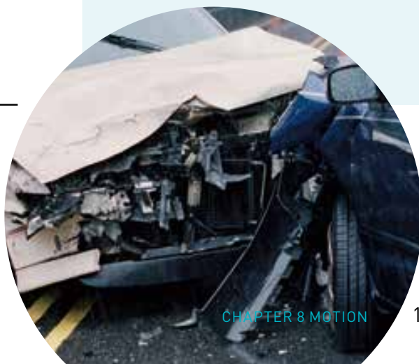
Figure 4 The rapid change in momentum as a result of a car crash can be seen in the crushed panels of this car.
