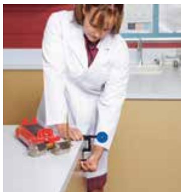
Figure 1 Clamping the pulley wheel to the desk
