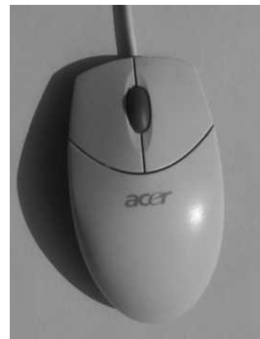
Fig 3.10 A typical mouse containing three buttons together with a scroll wheel.
