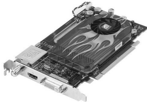
Fig 9.2 ATI All-in-Wonder includes plugs into a PCIe slot and includes DVI and HDMI interfaces.
