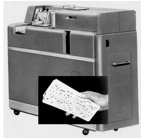
Fig 9.51 The IBM 533 Card Punch Reader with inset showing the punched cards used by the device.
