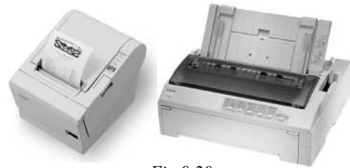
Fig 9.20 Epson's TM-T88 thermal receipt printer and FX-880 Impact dot matrix printer.
