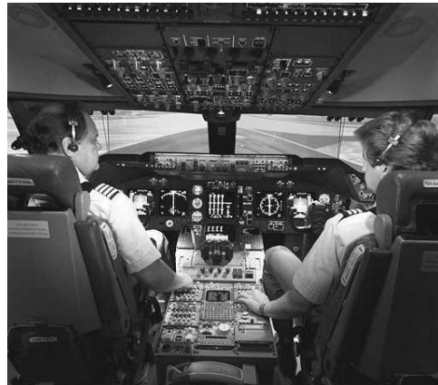
Fig 5.10 Boeing 747 flight simulator cockpit.
