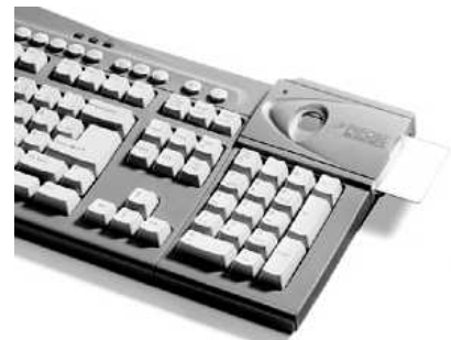
Fig 6.47 Precise Biometric's Precise 100SC integrates a fingerprint scanner, smart card reader and keyboard.
