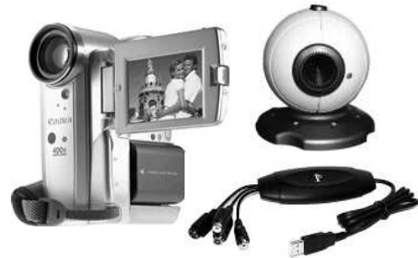
Fig 3.23 A digital camcorder, web camera and a video capture device.
