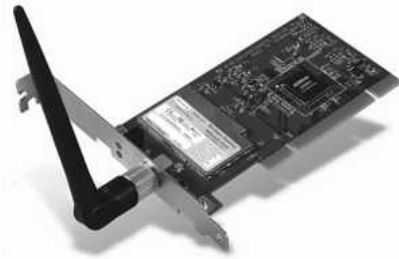
Fig 8.23 Belkin's 32-bit PCI wireless network interface card.
