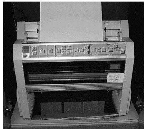
Fig 9.49 The Index Everest Braille embosser.
