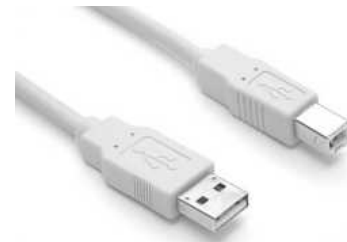
Fig 8.28 USB A and B type connectors.
