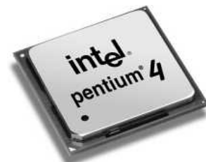
Fig 5.5 An Intel Pentium 4 central processing unit.
