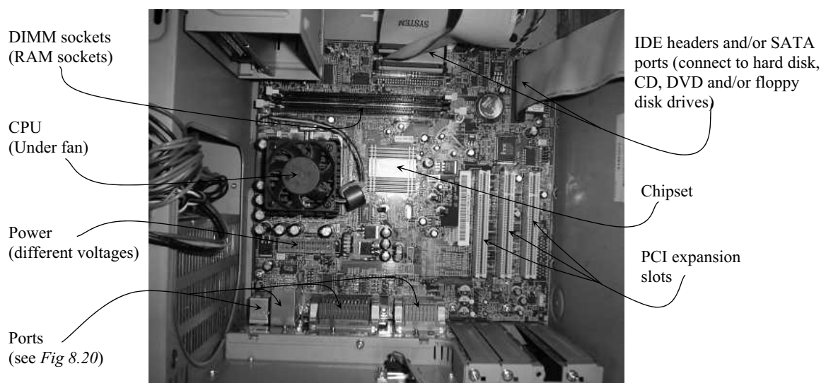
Fig 8.22 Major components on a typical motherboard.
