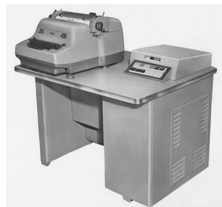
Fig 9.52 The IBM 838 Inquiry Station used for both input and printed output.
