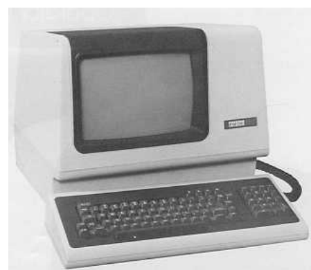
Fig 9.53 Digital Equipment Corporation’s VT100 terminal was released in 1978.
