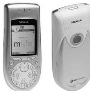
Fig 3.15 The Nokia 3650 contains a CMOS based digital camera.
