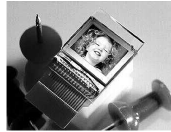
Fig 9.12 LCOS chip suitable for use in a mobile phone or PDA.
