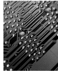
Fig 8.16 Bus lines on a motherboard.
