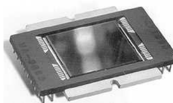
Fig 3.16 A CCD from a digital camera.
