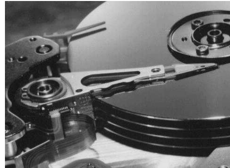
Fig 5.3 Internal view of a hard disk. The spinning disk platters and read/write head arms can be clearly seen.
