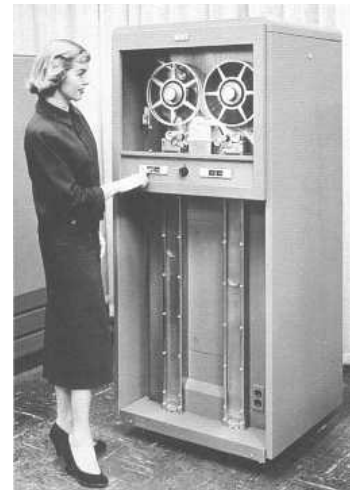
Fig 6.15 The IBM 726 magnetic tape drive released in 1952.
