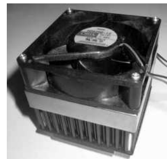
Fig 7.6 CPU fan and heat sink.
