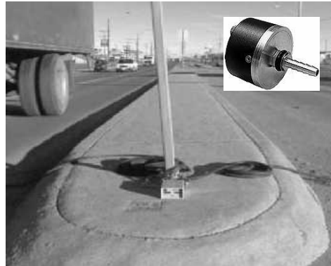
Fig 3.25 Air pressure based vehicle counter, with inset air pressure switch.
