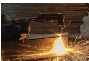
oxy-acetylene flame for cutting metal
