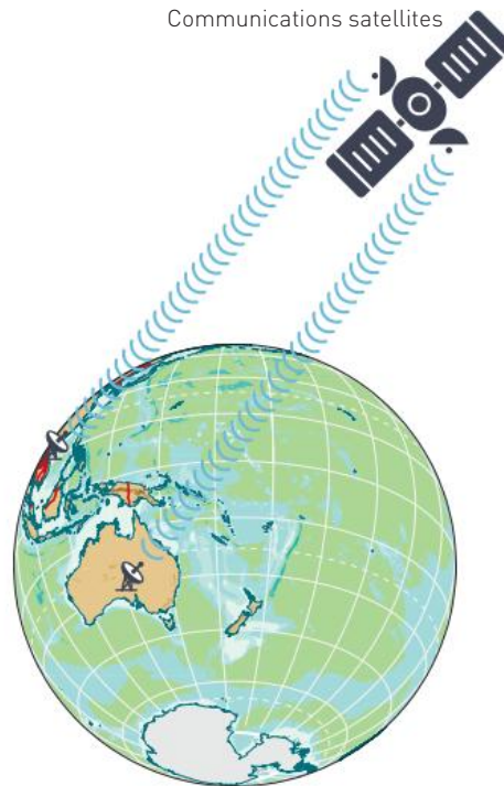
FIGURE 3.37 Communications satellites are placed approximately 37 000 kilometres above Earth's equator.
