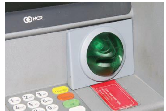
FIGURE 4.9 False card reader containing card skimmer added to an ATM
