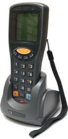
FIGURE 3.22 A handheld data-collection device is used for high-volume data collection, and features a touch screen, keyboard and number pad.
