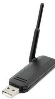
FIGURE 3.13 a A network interface card slots into the motherboard on a desktop computer. b A wireless adaptor can plug into the USB port on a desktop computer or notebook that does not have wireless capability.
